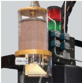
Tech-Sense Monitoring System provides the ability to run a night shift without the need for an attending operator. Should the cutting be disrupted, e.g. blocked nozzle, the machine will pause the program and send a text message to your cell phone.
