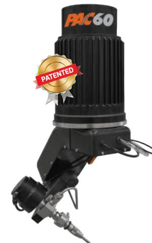
The PAC 60™ operating software incorporates the True Cut® algorithms data base, developed to determine the predicted taper at a given surface finish. This taper is then compensated for when cutting the part, anywhere from 0 to 60 degrees, giving you "Precision Angle Control" of any part that can be produced on an X-Y abrasive waterjet cutting machine.
