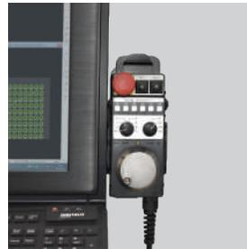
The MPG allows to manually wind forward or backward through a cutting path. This enables the operator to find the exact point along a cutting path from which to re-start cutting after a stoppage, or to accurately locate a pre-cut part.
