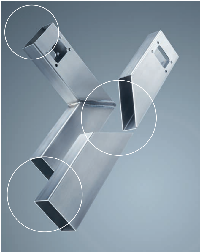
Conventionally welded from two single parts.
