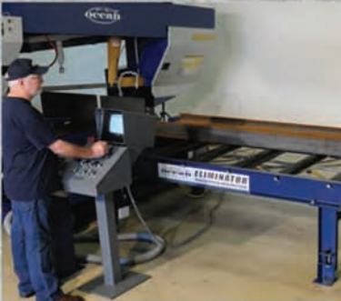
Cross transfer feeding to roller conveyor to band saw
