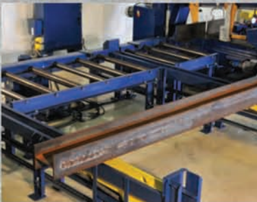
Cross transfer feeding to roller conveyors
