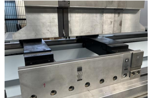
Sample picture: 4-axis back gauge incl. sensors
