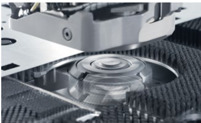
The descending die ensures scratch-free parts.
