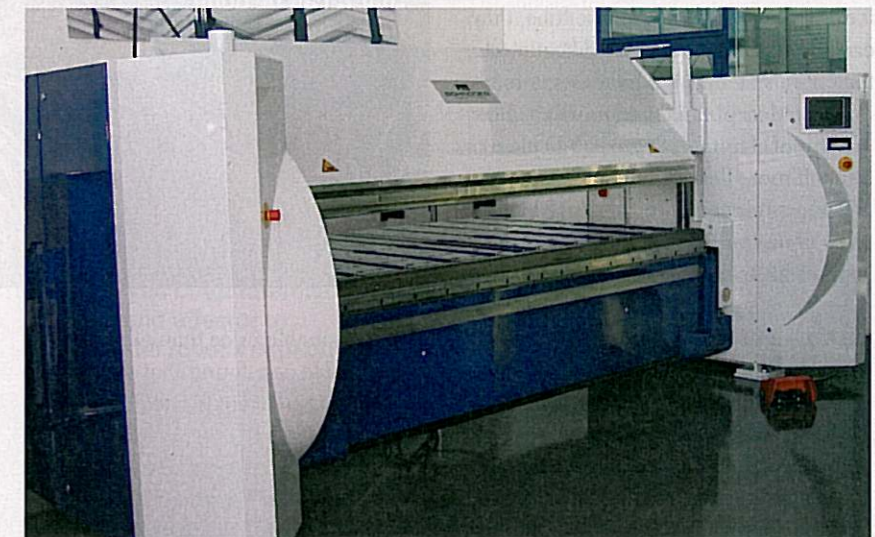
The folder’s backgauge holds the part, so the operator doesn’t have to. It results in less fatigue and increased part productivity.
